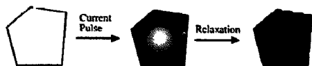
Fig. 5. Schematic representation of lithium activity in a graphite particle during intercalation. Depth of shading indicates lithium activity.
